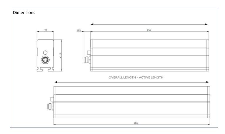
'T'M6 x 40 stud and flange nut. Two sliding brackets provided with each bar. Other stud lengths are available. Contact Static Clean for more information.
