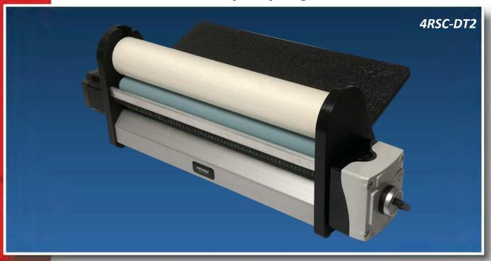
The Polymag® Tek Two-Sided, Desktop Sheet Cleaner (4RSC-DT2) offers big sheet cleaning capability in a small package. Driven Contact Cleaning Rolls (CCRS) remove contamination from the sheet and then transfer contamination to Adhesive Tape Rolls.
