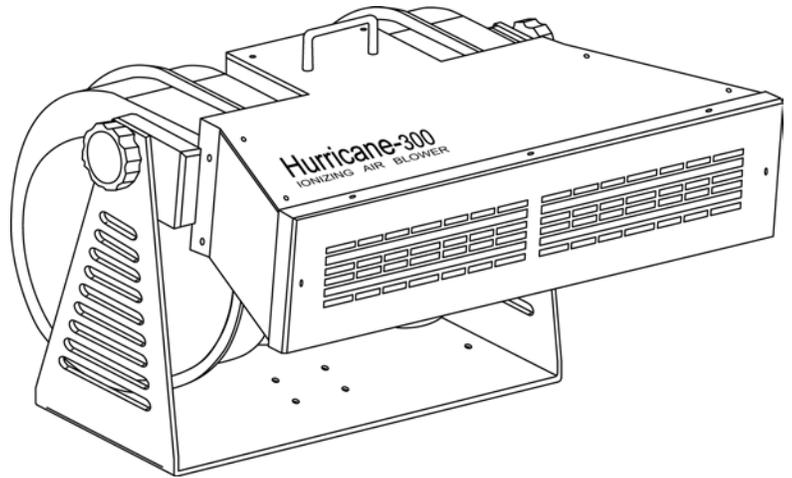
Most of the time, the best place to install any type of static control equipment is immediately ahead of the problem. For example, if an operator is getting shocked from a rewind roll, then the ionizer should be placed so that the last thing the material passes before it winds onto the roll is the ionizer.
